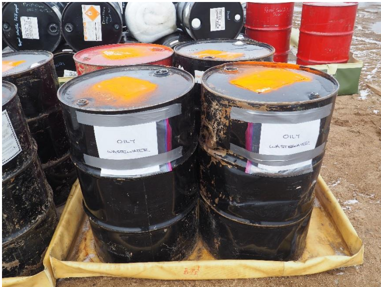
Drums at Satellite Bay containing water pumped from berms and drip trays.
