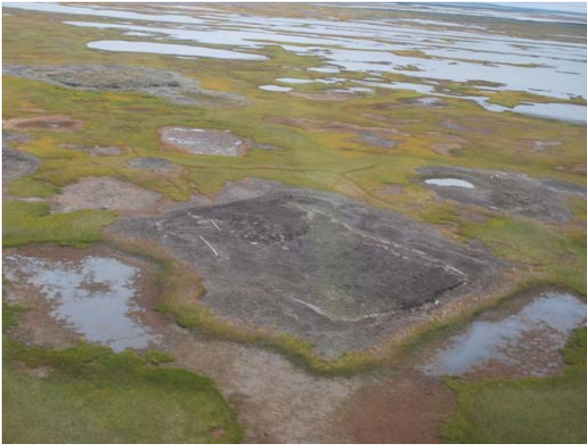
Figure 1 Aerial overview of drill sump, water ponding around the sump edges. Some subsidence on the sump cap, August 24, 2011.
