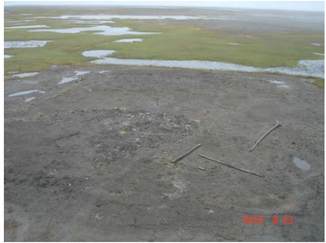
Figure 2 Drill sump cap with subsidence and ponding present. Poor vegetation growth, coverage of <10%, August 23, 2010.
